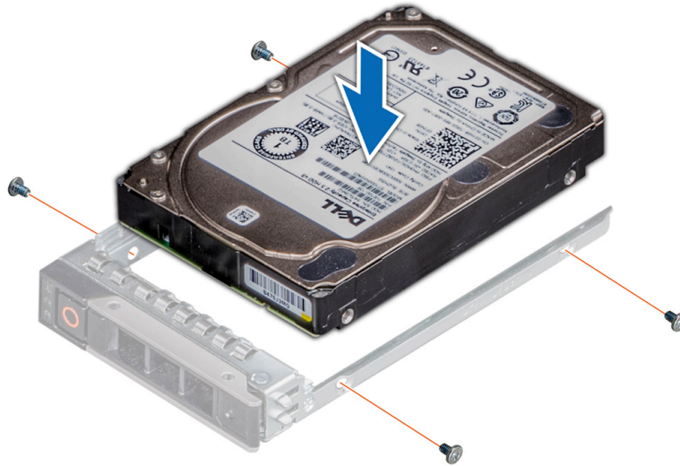
Figure 59. Installing a drive into the drive carrier
